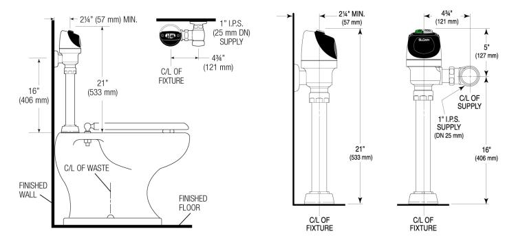
The Model 8113 valve is designed for installations where toilet seat with covers are being used.
